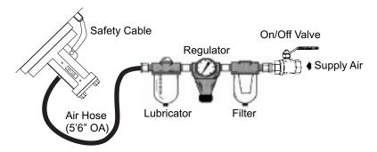
The vibrator should be installed no further than 15 feet from the on/off valve and lubro-control unit. The NPT size of the Lubro-Control Unit and On/Off Valve should match the NPT of the vibrator air inlet in single unit installations. When more than one vibrator will be controlled using the same valve and lubro-control unit, the NPT Size of each component should be increased by 1/4" for each vibrator added to the system.
